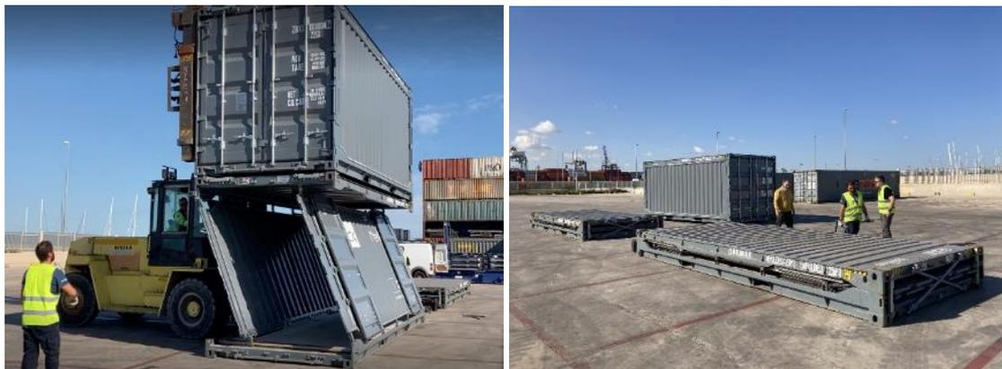
Figure 9. Zbox folding and unfolding trials at depot
